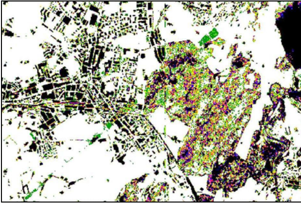
Fig 2: 10 x 10 m laser point density calculated on a DTM-AV extract (1 pixel = 10 x 10 m)
