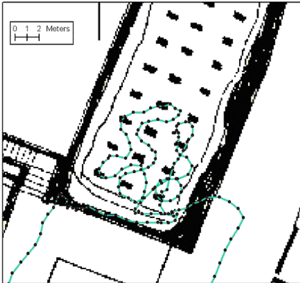
Fig. 8 – A complex path surveyed by BT-GPS EMTAC
