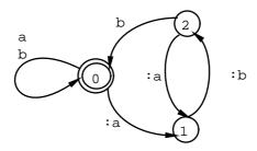
Figure 2. Transducer implementing  $\varepsilon \rightarrow ab / b$
