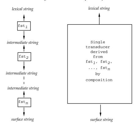
Figure 9: Replacing a cascade by a single transducer
