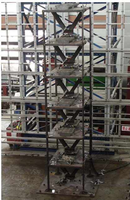
(a) Six-Story Laboratory Structure
