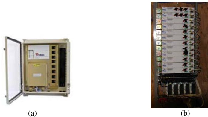
Figure 3 Evolution of MDU Common ONT. (pictures not to scale)
