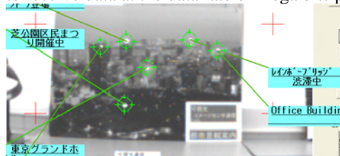
Figure 4: Application Example of Visible Light Communication using Image Sensors as Receivers [7]
