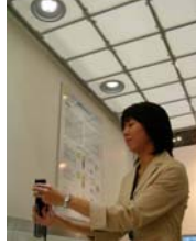
Figure 3: Indoor Location Detection using Cellular Phones and Visible Light LEDs [6] Typical applications of such location-based services are shown in Figure 3, where a user uses a cellular phone with a visible light sensor, which detects signals from an LED light. This application is especially useful indoors because GPS receivers do not work well indoors even though they work well outdoors.
