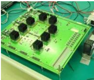
Fig. 2. FPGA board for emulating LDPC DEC.
