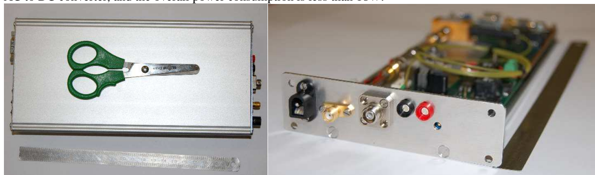
Fig. 1. Photograph of the implemented module: QDa-MLLD laser source overall picture (left), inside picture showing the electronic card (right)
