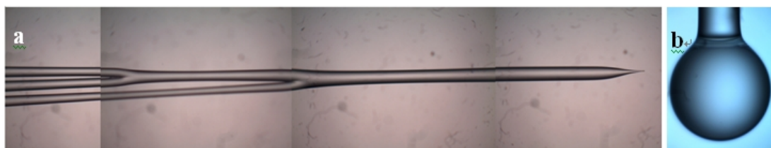
Fig. 2: (a) A typical 3x3 coupler made and tip-shaped by the splicer. (b) The ball lens made of a coreless silica optical fiber.
