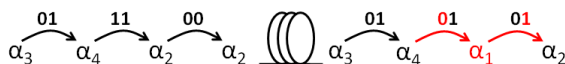
Fig. 1: Principle of transmission error on QPSK systems using differential encoding ( \alpha_1, \alpha_2, \alpha_3, \alpha_4 are the four states of the QPSK constellation)
