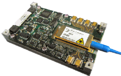
Fig. 2(b) Transmitter integrated into the TTA format
