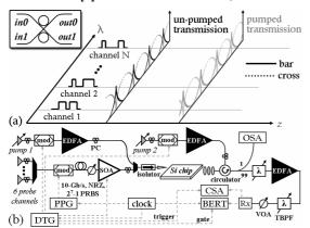
Figure 1: (a) Diagram of multi-wavelength packet structure and switching scheme with inset of device and port labels. (b) Experimental setup schematic.
