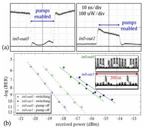
Figure 2: (a) CSA traces (16-point average) showing the switching envelope for two labelled paths. (b) BER curves representing these paths under dynamic and static states of the switch with waveform insets.
