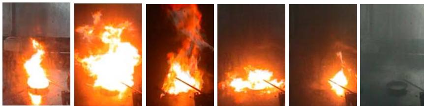
Fig.11. Test results of fire suppression with different water flow rates: (a) gas operation pressure is 0.20MPa, (b) distance between the fire and nozzle is 2.0m
