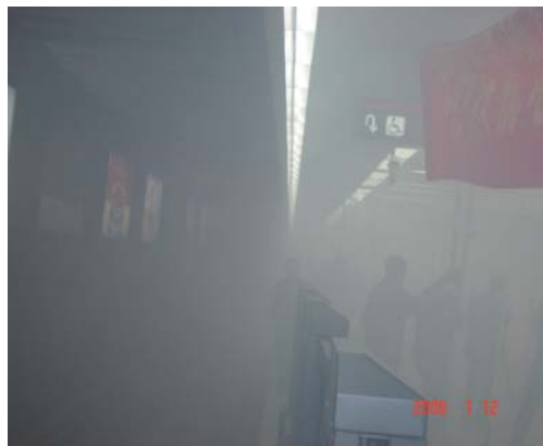
Fig.7. hot smoke test: north end of platform (the hot smoke source was at the center of the platform)
