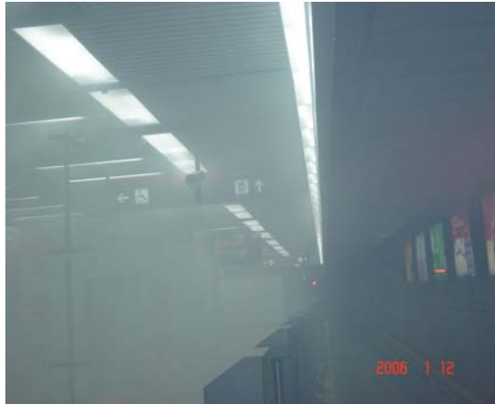
Fig.6. hot smoke test: south end of platform (the hot smoke source was at the center of the platform)
