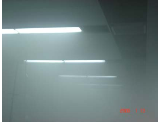
Figure.3. smoke movement in concourse during hot smoke test (fire source at the center of the concourse)
