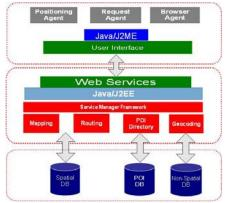
Figure2. Location Based Service Architecture
