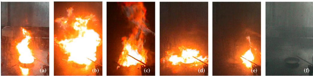
Fig. 12. Diesel pool fire behavior before and after the injection of water mist (gas pressure: 0.30 MPa, distance: 2.00 m, water flow rate: 80 kg/h): (a) before water mist injected, (b) water mist injection started, (c) 6s after water mist injection, (d) 11 s after water mist injection, (e) 14 s after water mist injection, (f) 16 s after water mist injection.
