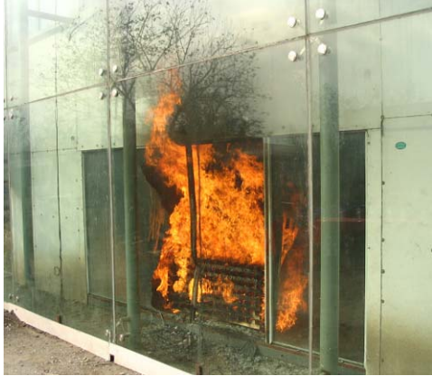
(a) flame spread into the cavity;
