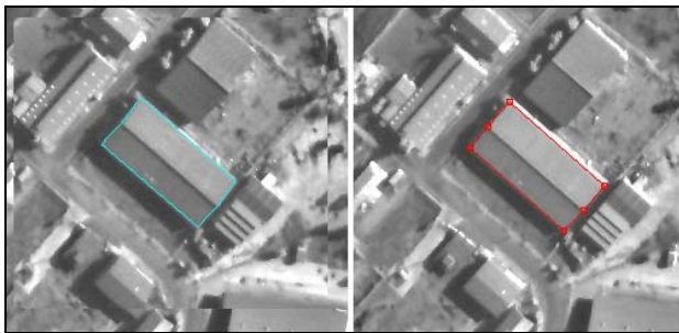
Figure 2: An extracted building from an IKONOS stereopair. The left building is measured manually and the right one is matched automatically.
