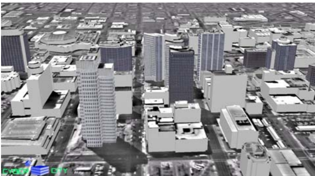
Figure 8. 3D city model generated with CC-Modeler from Quickbird images. Visualization in TerrainView by ViewTec (Courtesy of Eurimage S.p.A., Italy).
