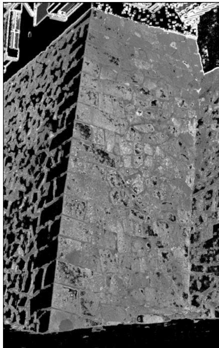
(a) Threshold=0.005m Fig.9 Classified Result by Flatness
