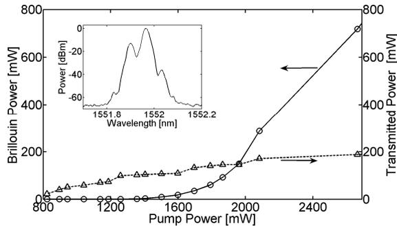
Figure 3: Backscattered and transmitted powers as a function of the 2-m long chalcogenide fiber input power. Inset: Typical Brillouin spectrum.
