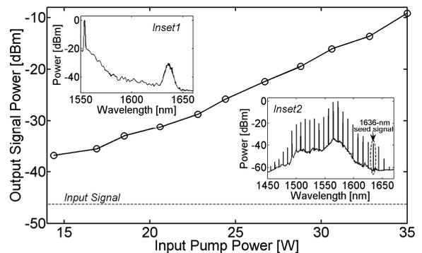
Figure 5: Output 1636-nm seed signal power as a function of input 1553-nm pump power. Inset1: Spontaneous Raman scattering for an input pump power of 80W. Inset2: Frequency-comb used to generate the 1636-nm seed signal.
