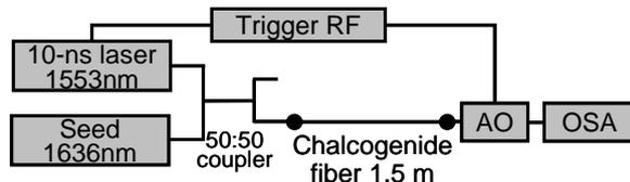
Figure 4: Experimental set-up for Raman characterization.
