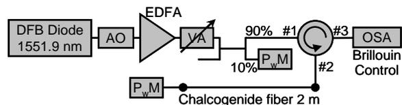
Figure 2: Experimental set-up for Brillouin characterization.
