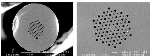
Figure 1: Pictures of the section of the  $Ge_{15}Sb_{20}S_{65}$  chalcogenide microstructured optical fiber.
