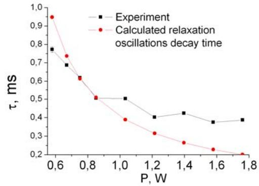
Figure 5: Dependence of  $\tau$ -parameter on pump power
