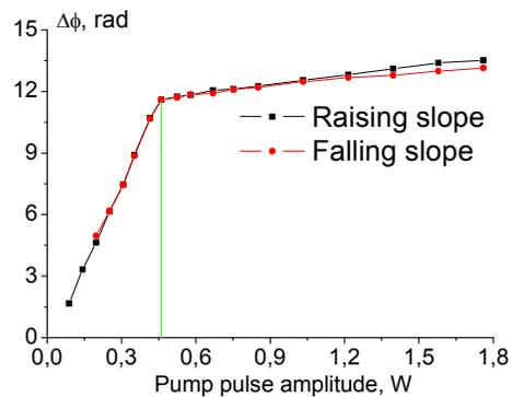
Figure 6: Dependence of full phase shift on pump power. The laser threshold is denoted by green vertical line.
