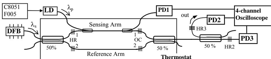
Fig 1: Experimental setup: LD – pump radiation ( $\lambda_p = 962 \text{ nm}$ ), DFB – source of probe light ( $\lambda_s = 1564,8 \text{ nm}$ ), C8051F005 – microcontroller, PD – photodetectors, HR, OC – fiber Bragg gratings.
