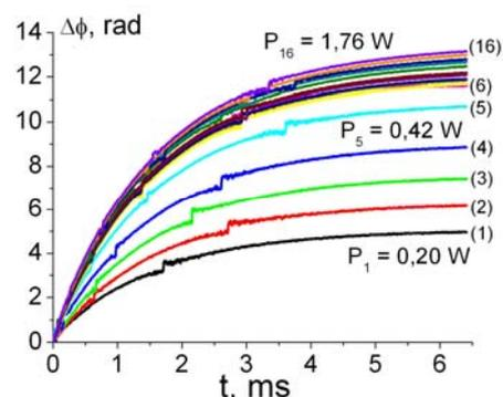
Fig 3: Dependence of phase shift on time after pump pulse switched off.
