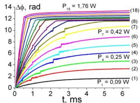
Fig 2: Dependence of phase shift on time after pump pulse switched on. Pulse amplitudes alternates from 0.09 W to 1.76 W
