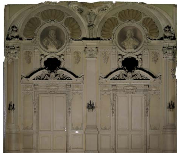
Fig. 10 – The true orthophoto of the northern wall.
