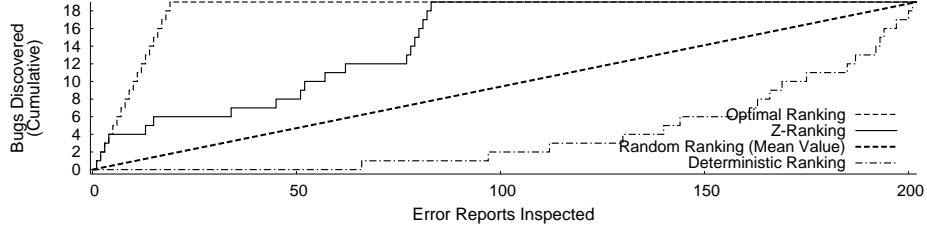
Fig. 2. Results of inspecting Linux spin-lock error reports. Z-ranking uses p_0 = 0.21 , with 175 populations created by \mathcal{G} , and 14 equivalence classes. 202 reports inspected, with 19 real bugs. Within the first 21 ( \sim 10\% ) inspections, z-ranking found 3 times more bugs than the expected number found using random ranking. When using the no-success heuristic, we inspect only the first 83 reports, discovering all real bugs.
