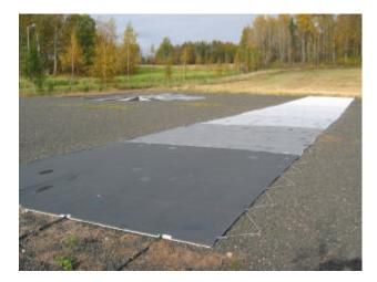
Figure 2. Targets at the Sjökulla photogrammetric test field in Kirkkonummi arranged for a digital aerial camera test. (Photo 4 Oct. 2004 by H. Kaartinen).
