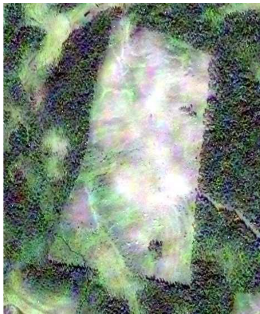
Fig. 2. Logging area in the north of Russia. Fusion of EROS and SPOT 4, 2006, resolution 2 meters.
