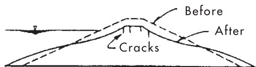
Fig. 5. Typical earthquake-induced damages to earth dams.
