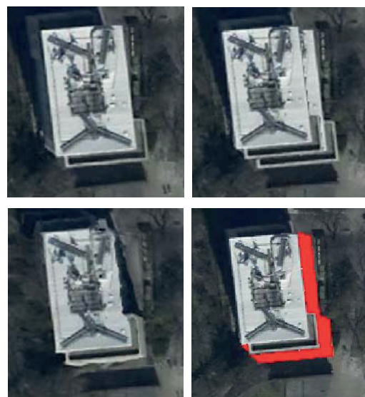
Figure 6: (a) Orthophoto (above-left) and (b) Ghost effect (above-right), (c) Visibility test result (below-right) and (d) True orthophoto (below-left)
