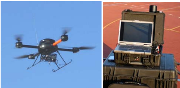
Figure 2: Micro UAV (microdrones md4-200) with digital RGB camera (left) and portable ground control station (right).
