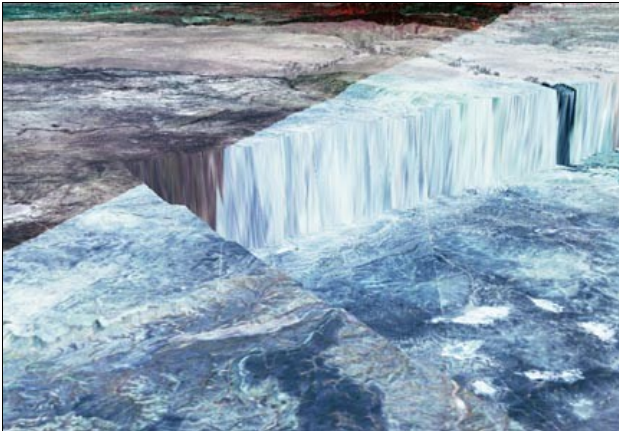
Figure 18 : a step between no-data terrain areas and terrain areas, with 120x terrain accentuation
