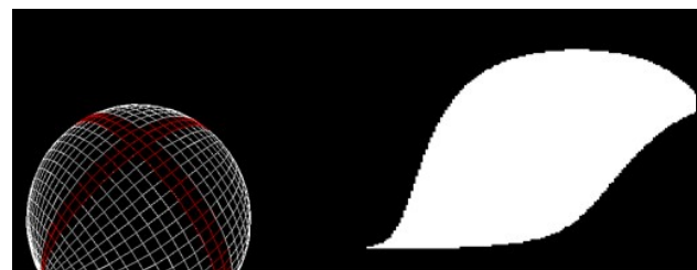
Figure 4. Intersection of a frustum and a WGS84 ellipsoid
