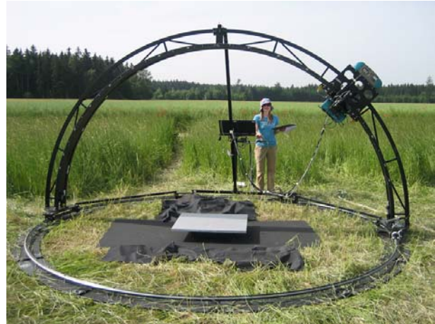
Figure 1. Dual field-of-view goniometer system FIGOS
