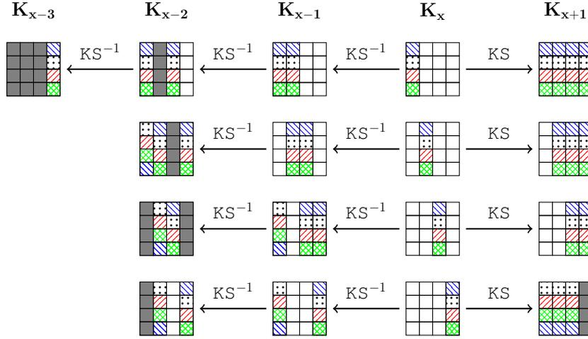
**Fig. 7.** Backward and forward truncated differential transitions through the AES-128 key schedule when only one column is active in  $K_x$ . The propagation of each active cells in  $K_x$  can be traced using the same shade pattern. The white cells represent inactive bytes, while the gray cells can be either active or inactive.
