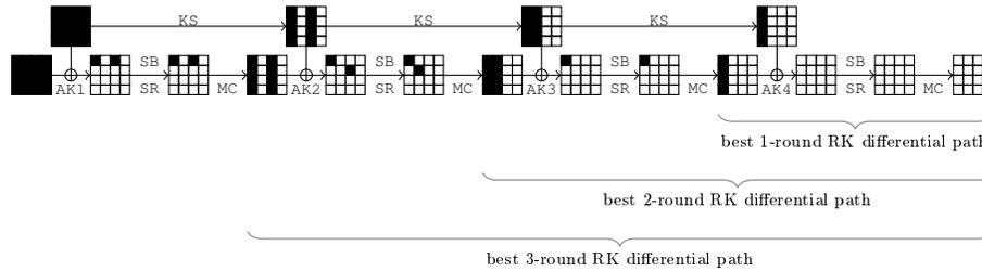
Fig. 5. Example of best possible 1/2/3/4-round related-key truncated differential paths for AES-128. The black/white cells represent active/inactive bytes.
