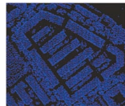
Fig. 2 Non-ground points after filtration ground points
