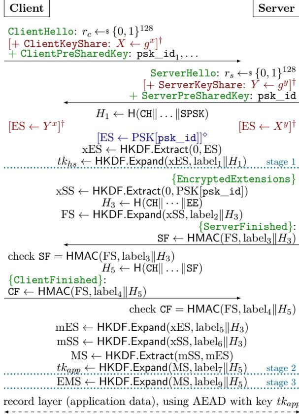
Figure 2: The PSK and PSK-(EC)DHE handshake protocol in TLS 1.3 `draft-ietf-tls-tls13-10`. See caption of Figure 1 for notation. Messages/computations only in PSK-(EC)DHE are marked with  $[ \dots ]^\dagger$ . Messages/computations only in PSK (without (EC)DHE) are marked with  $[ \dots ]^\circ$ . The key schedule is identical to that of Figure 1, except that no RMS is derived.
