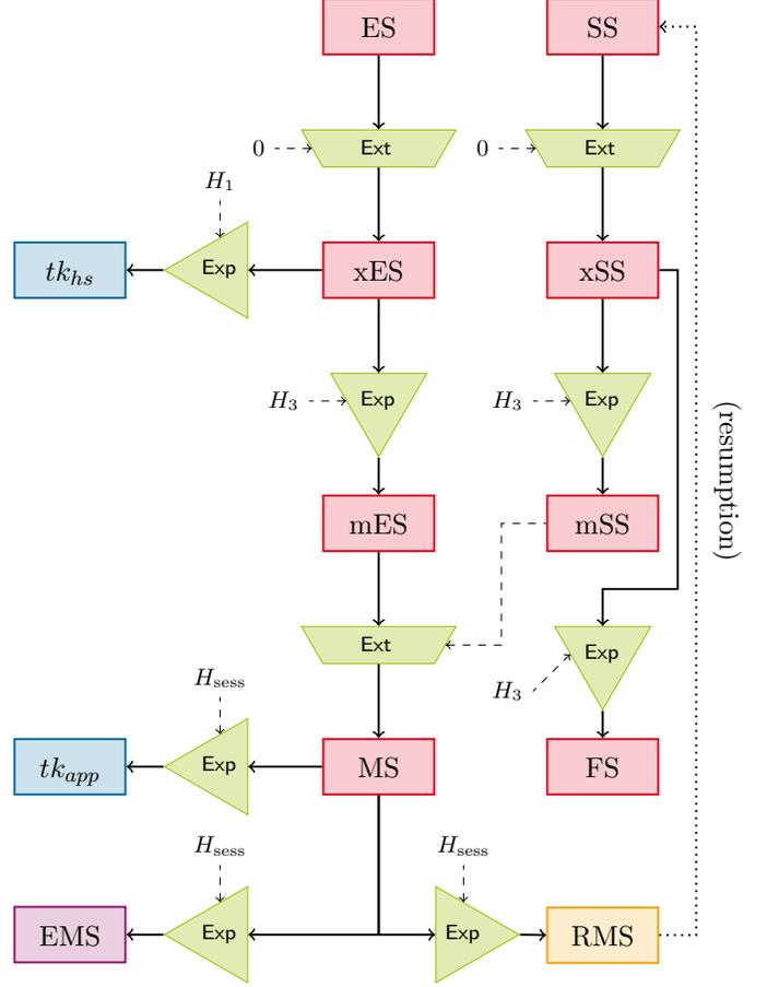
Figure 1: The full (EC)DHE handshake protocol in TLS 1.3 draft-10 (left) and its key schedule (right).
