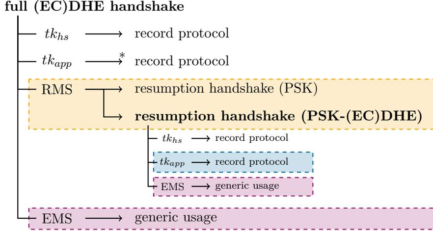
Figure 3: Illustration of the composition result applications in our analysis of the TLS 1.3 `draft-10` full and pre-shared key handshakes. Derived keys are connected to the handshake by solid lines, their usage in protocols is indicated by an arrow. Dashed boxes indicate an application of the composition result to the usage of a specific derived (final) key in the subsequent symmetric-key record or resumption handshake protocol.
