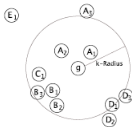
Figure 5. Visualization of the KNN classification. The k=7 nearest neighbour are used. The object g is assigned to the class B
