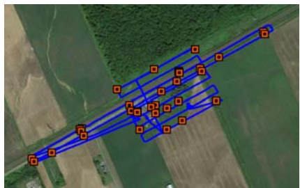
Figure 3: GCP distribution for the block and railway corridor viewed in Google Maps
