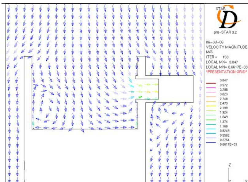
Fig. 10(a). Velocity vectors for SF 6 release flow rate of 10 L/min, venting flow rate of 313 L/min (Case 1).
