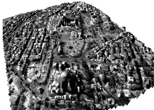
Figure 6. Extract of 3m surface model, draped with panchromatic ortho-image for photorealistic visualization.
