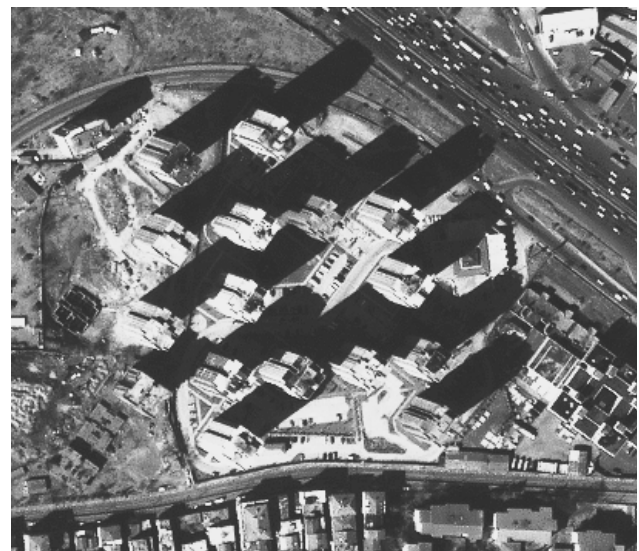
Figure 1. Extract of original 11-bit Ikonos image, illustrating an area with high buildings. There is very little contrast within the shadow areas, leading to mismatches during the image matching process.
