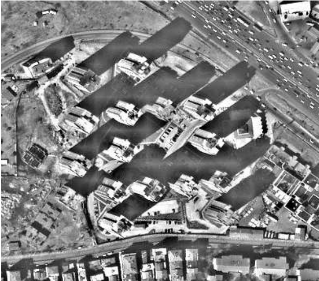
Figure 2. Extract of Wallis-filtered 11-bit Ikonos image. The radiometric filter enhances the existing texture patterns locally, leading to optimization of the contrast in the shadow areas.
