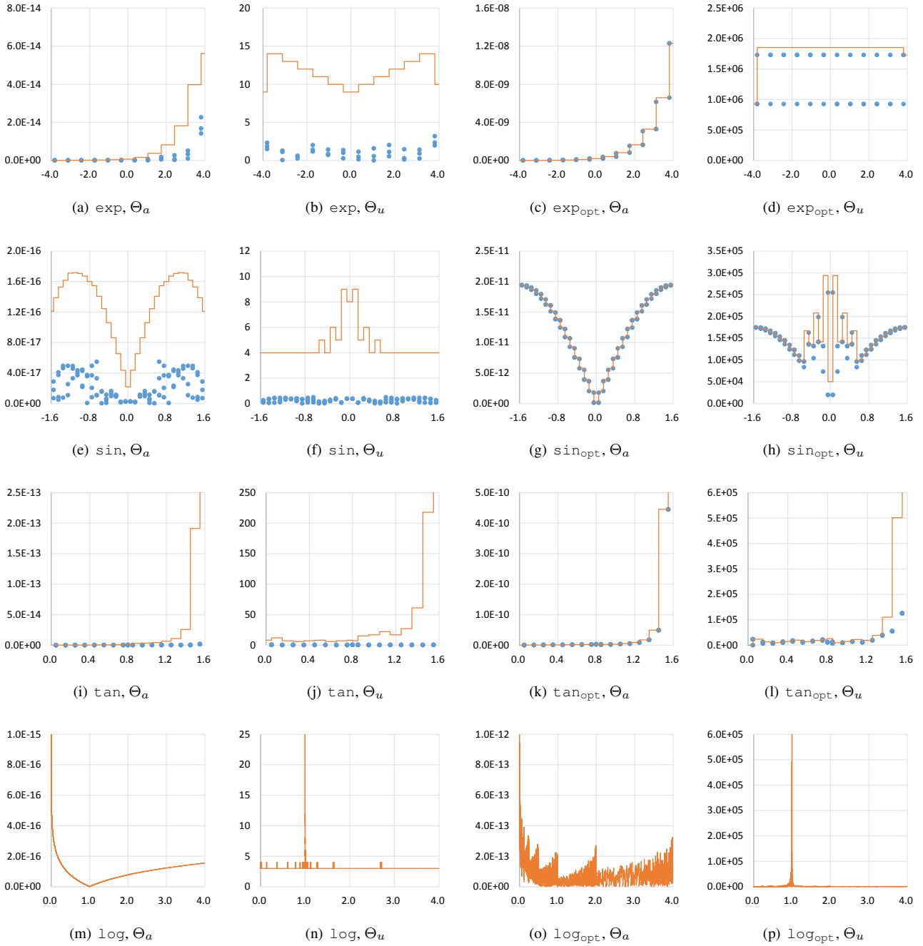
Figure 7. Each graph shows a bound on precision loss between an implementation and the mathematically exact result. For example, (a) plots a bound on absolute error between \exp(x) and e^x as a function of x . The brown lines represent the bounds obtained from symbolic abstractions and the blue dots signify the errors observed during explicit testing on inputs in \hat{H} .
