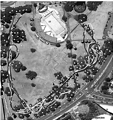
图 6 重载卫星图的 SLAM/GPS 与 GPS 定位结果 Fig. 6 SLAM/GPS and GPS positioning results with environment satellite image
