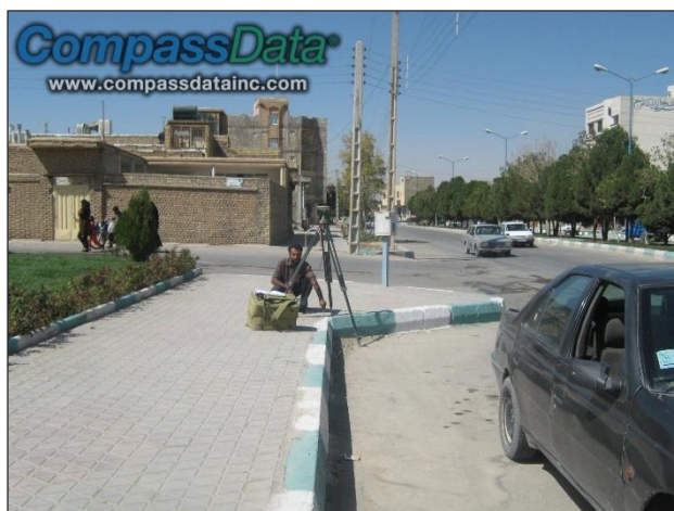
Figure 7. Elevated Curb as GCP
