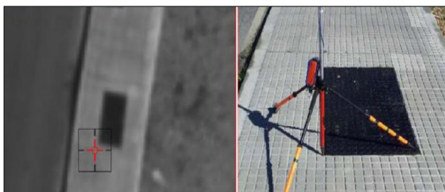
Figure 5. This black vault is visible on high resolution imagery, but will blend in with lower resolution imagery by satellites.
