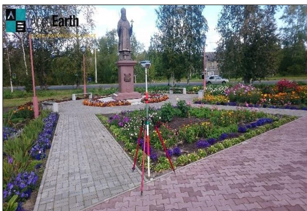
Figure 1. Clear Photo-identifiable GCP
