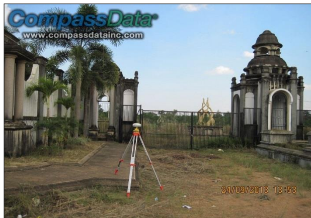
Figure 2. Difficult Photo-identifiable GCP
