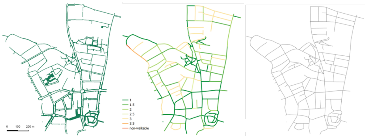
Figure 1. Footpath network 1 (left) comprising car traffic free paths only; footpath network 2 built from walkability rated streets (middle, the colour coding is explained in Table 1); and the un-rated street network (right). (Data sources: Amt für Geoinformation Kanton Solothurn 2016; Direktion Öffentliche Sicherheit, Stadt Olten)
