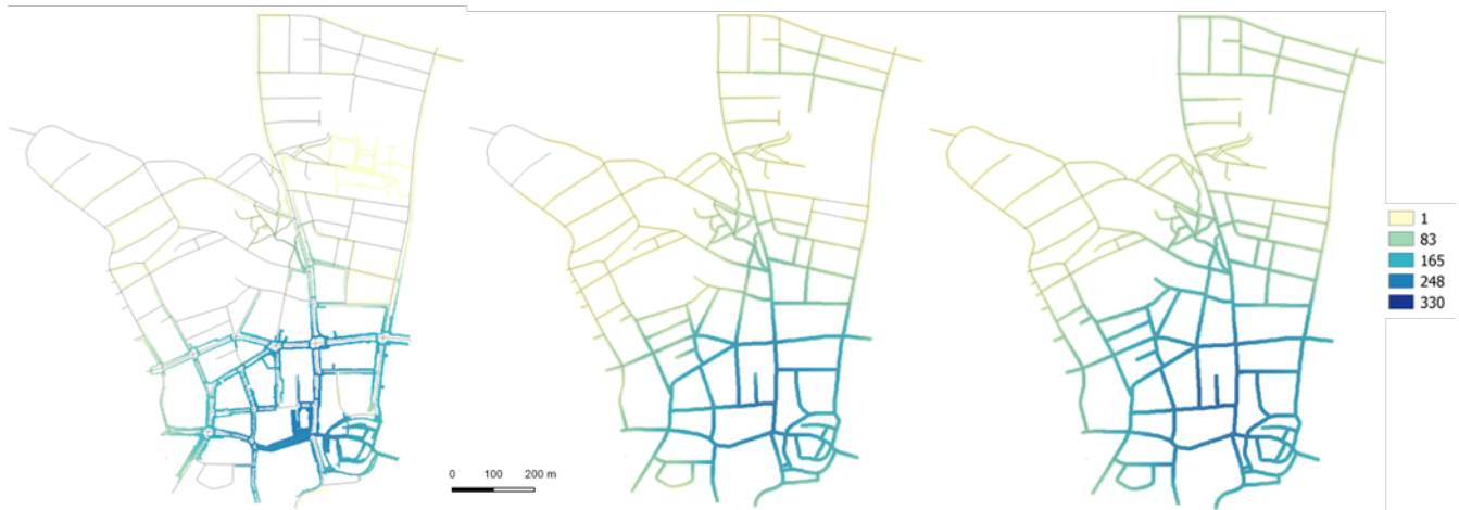
Figure 5. Access-to-destination maps (number of accessible amenities within 400m) calculated based on footpath network 1 comprising car traffic free paths only (left); based on footpath network 2 built from walkability rated streets (middle); and based on unrated street network (right). (Data Sources: Amt für Geoinformation Kanton Solothurn 2016; Direktion für Öffentliche Sicherheit, Stadt Olten)
