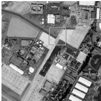
Fig.3 Navy airfield AVIRIS data's false color composite image in San Diego, California, United States(Band 28,19,10)
