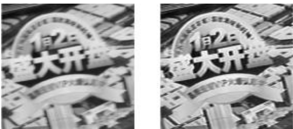
(a) 可见光运动模糊图像 (b) 文中方法复原结果 (a) Motion visible light blurred image (b) Restoration result with the proposed method
