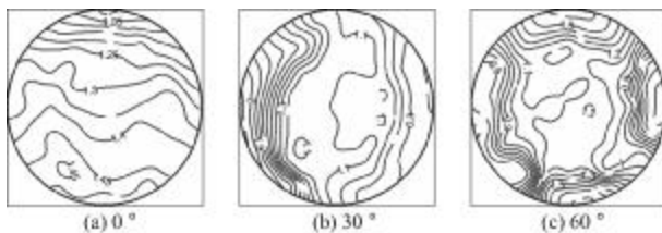
Fig.14 Mean wind pressure coefficients of the reflector in different wind directions for 5^\circ pitch angle
