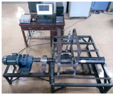
a. 滑动摩擦系数测试装置原型 a. Picture of device for measuring sliding friction coefficient
