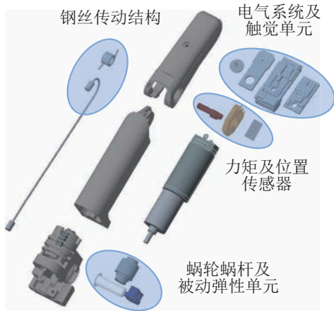
图1 智能假手指 Fig.1 Intelligent prosthetic finger
