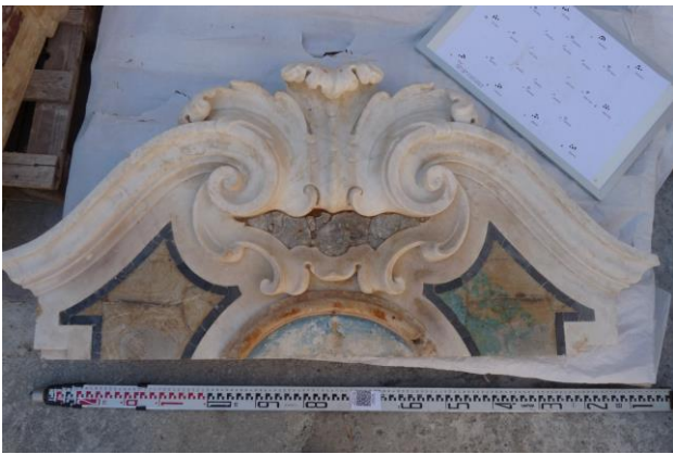
Figure 6. A typical image (piece #85). Notice the linear rod, the QR-Code with references and metadata and the calibrated grid.
