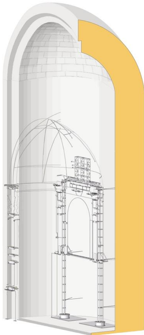
Figure 10. View of the mounting structure positioned in the apse.
