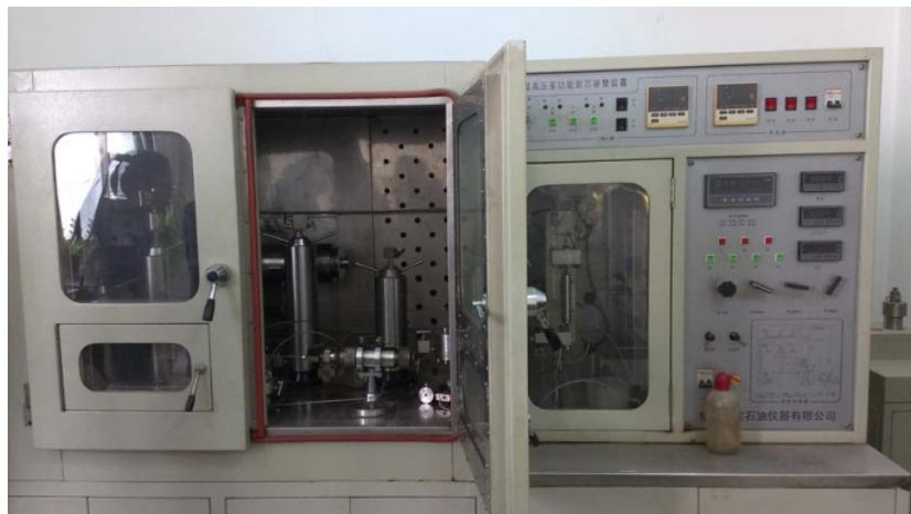
Fig. 4 Core displacement device of indoor simulation experiment
