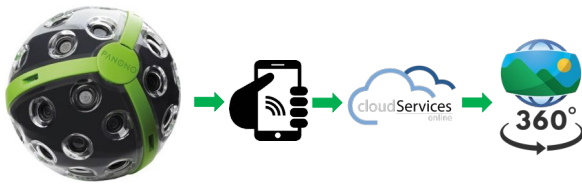
Figure 1. The Panono 360° with a schematic representation of the workflow used to create panoramas.
