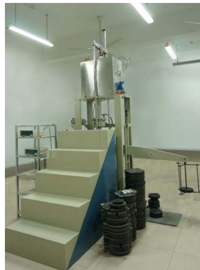
图 5 大型高压固废仪 Fig.5 Large-scale high-pressure solid waste compression apparatus
