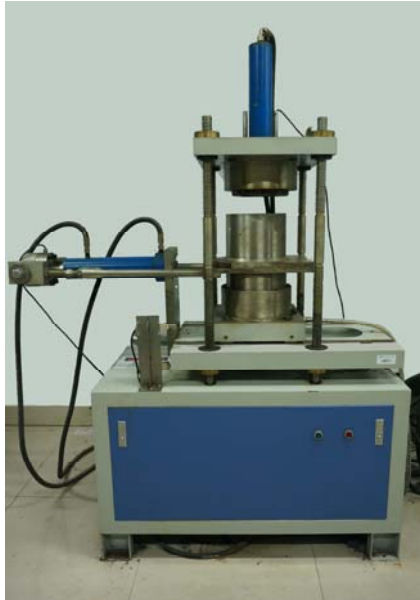
图 6 SYTL - 2000 型双向液压伺服位移剪切联合测定仪 Fig.6 SYTL - 2000 Bidirectional hydraulic servo displacement and shear combined apparatus
