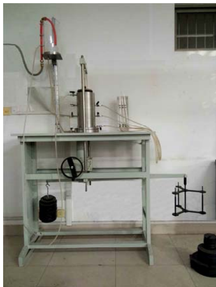
图 7 压缩渗透联合测定仪 Fig.7 Compression and permeability apparatus
